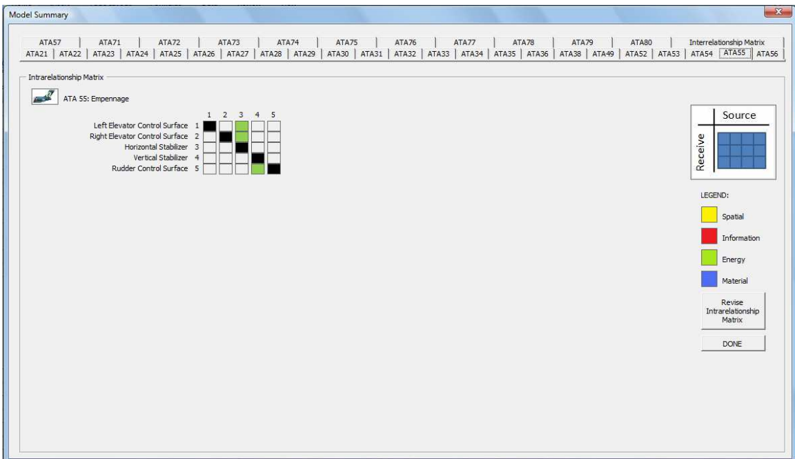
Figure B.22: DSM Model for ATA55 Subsystem of the Notional Aircraft System
