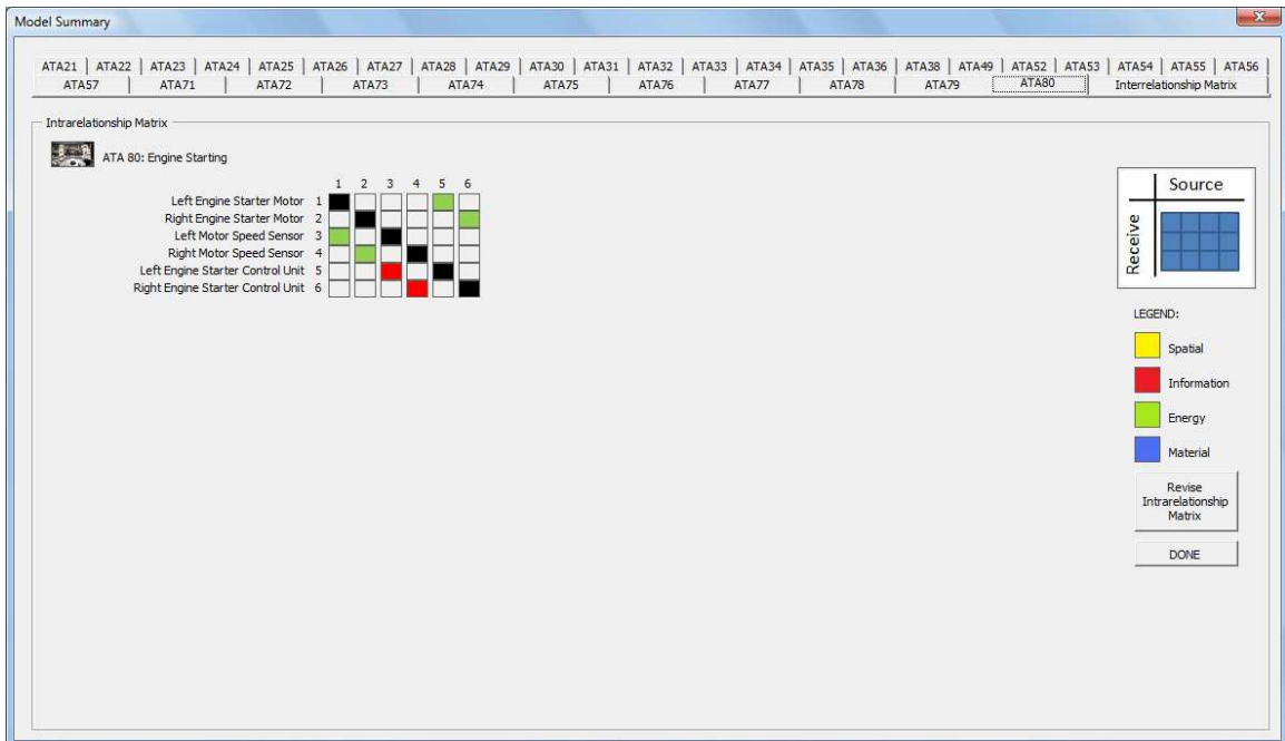
Figure B.34: DSM Model for ATA80 Subsystem of the Notional Aircraft System
