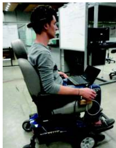
Fig. 14. Healthy user controlling the powered wheelchair with the BCI using Gestures with the Cognitive Suite (picture taken on Dec 20 th 2012).
