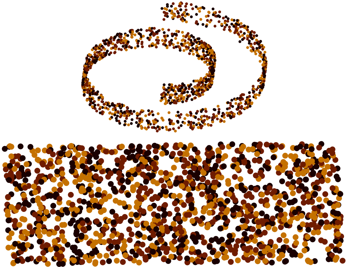
Figure 42: Top: Three classes laying randomly on a swiss roll. Bottom: After unfolding them with MVU the classes are not linearly separable. Isometric Separation Maps managed to map this manifold in a 12-dimensional space such that the classes were linearly separable by 3 hyperplanes. The optimization algorithm terminated with feasibility error 0.4% for 5-neighborhood distance preservation, while 99.83% of the points were correctly classified. The goal of this experiment was to verify experimentally that ISM can lift any strange dataset to a high dimensional space, such that classes are linearly separable
