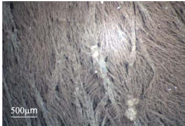
Figure 3.18: Optical microscope image of 2vol% aligned acicular nanomagnetite embedded in DP5.1 resin. Heating
