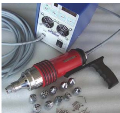
Fig. 14. The new ultrasonic system UltraPeen® with easy replaceable working heads for underwater ultrasonic peening
