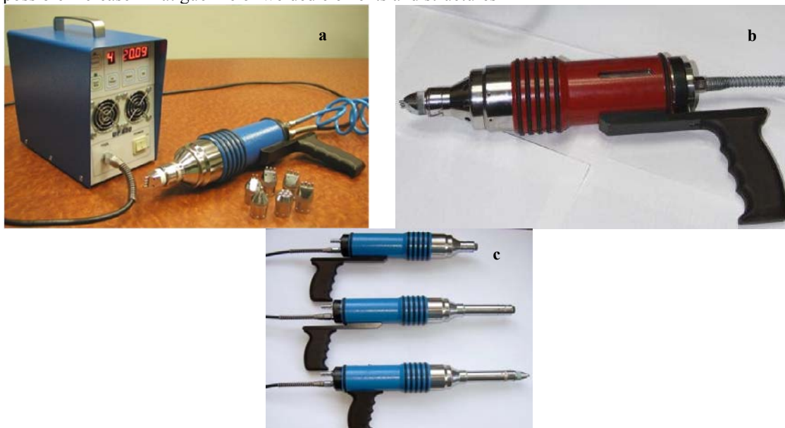
Fig. 6. Basic ultrasonic peening system for fatigue life improvement of welded elements and structures (a) and the underwater peening instrument (b) and various modifications of the basic peening tool (c)
