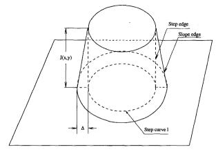
Fig. 1. Interpretation of integral by impulse function when there are step edges in the image.
