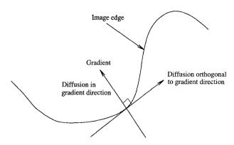
Fig. 3. Orthogonal decomposition of anisotropic diffusion.
