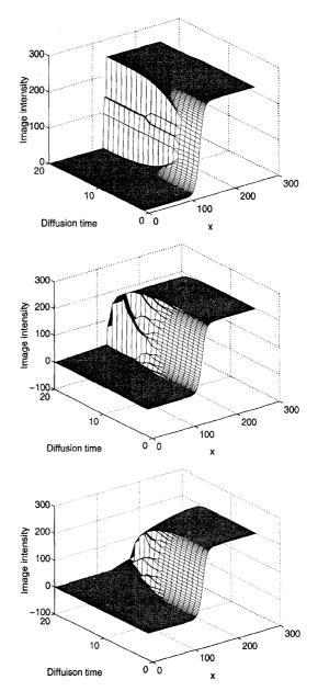
Fig. 6. Evolution with time of a slice along the x axis of the smooth sigmoid image when it is processed by anisotropic diffusion. Note that the indexes in the "Diffusion time" axis are the powers of 2. Top: Perona and Malik's diffusion. Middle: extended version of the diffusion scheme previously developed by the authors. Bottom: diffusion scheme that does not have step images as its stationary points, though step images appeared anyway.
