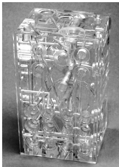
Fig. 1. Example-workpiece with intersection boreholes, Co. HELLER
