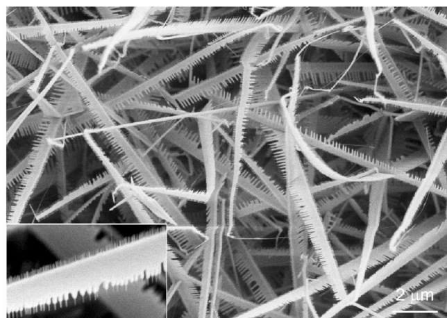
FIG. 1. Scanning electron microscopy image of the double-sided “comblike” structure grown by a solid-vapor process.
