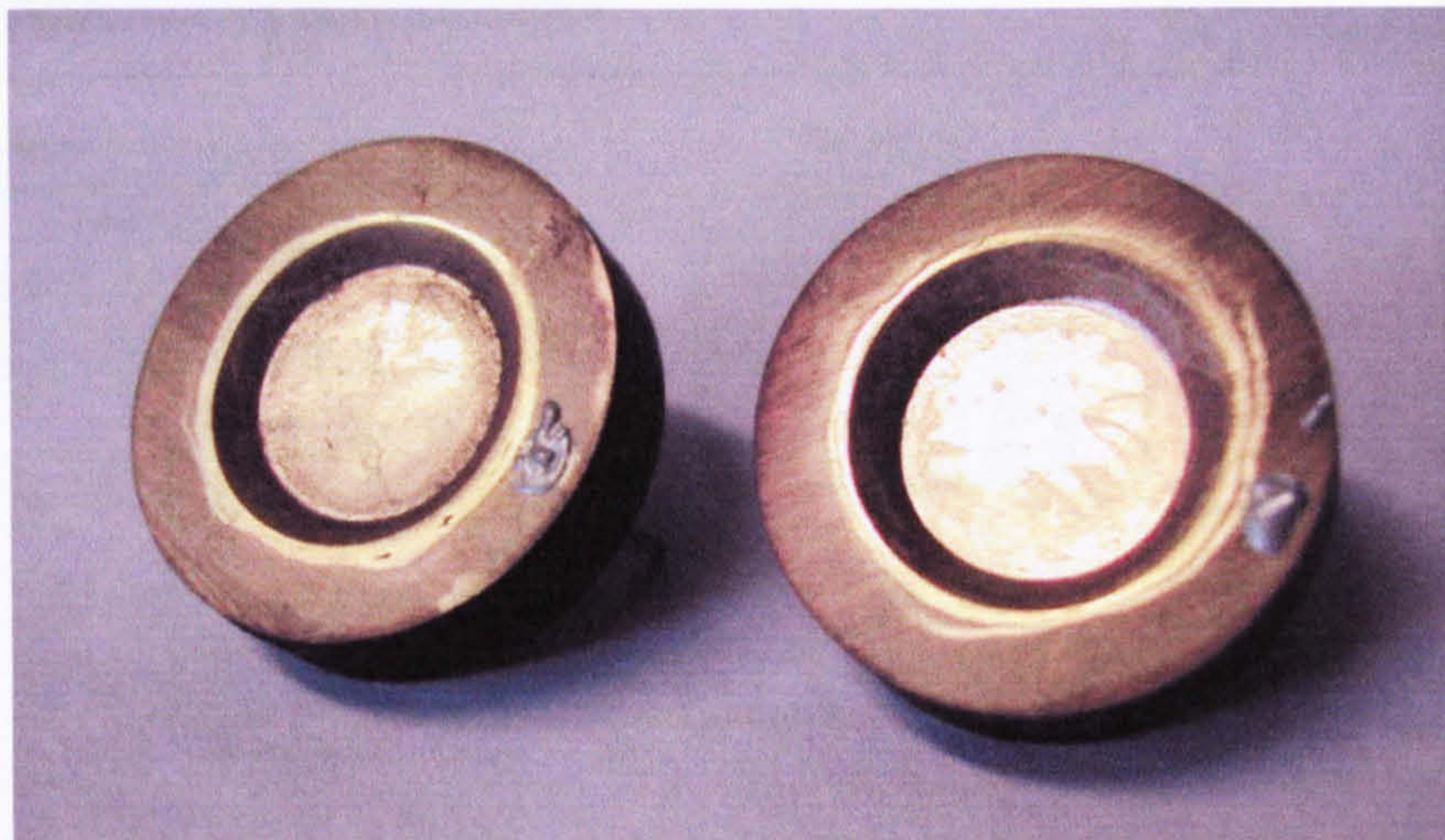
Figure 4.6 – Photograph of two MSL transducers showing membranes
