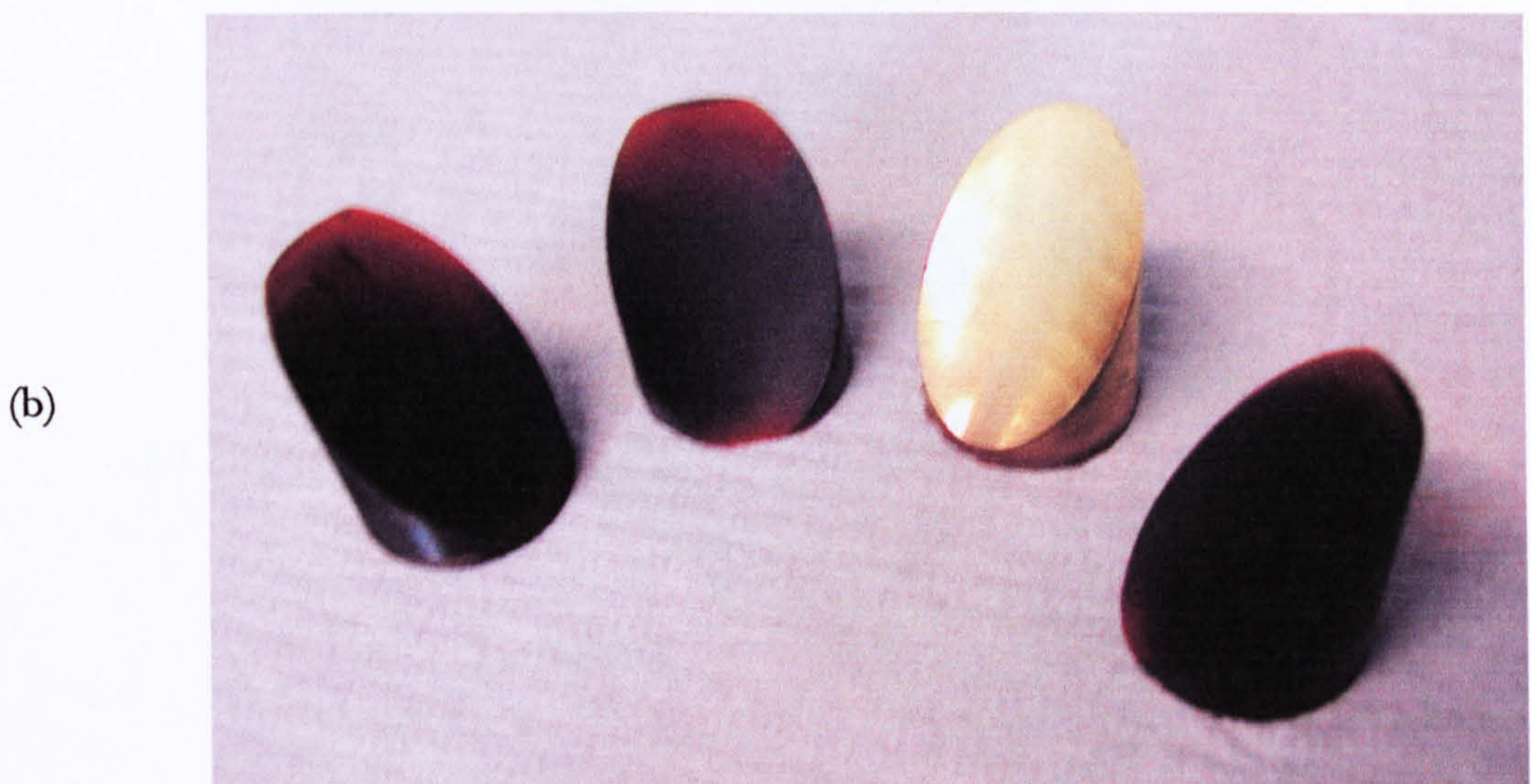
Figure 6.10 – (a) Comparison of the profiles of two different parabolic mirrors and (b) a photograph of some fully-focused parabolic mirrors produced using microstereolithography
