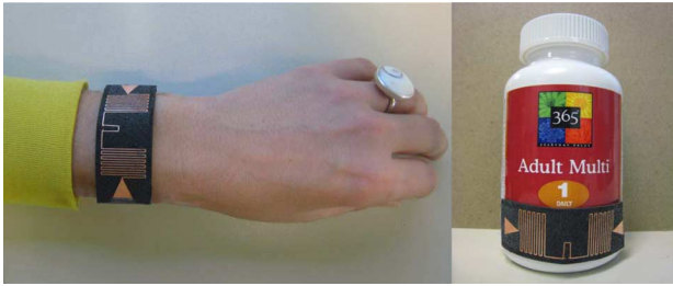
Fig. 10. Embodiments of the conformal RFID tag prototype in the applications of wireless health monitoring and pharmaceutical drug bottle tracking.
