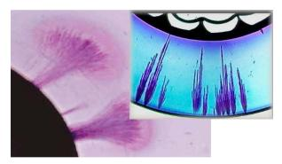
**Figure 3** Water Trees Growing from the Inner (bottom) and Outer (top) Semiconductive Screens
