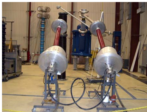
Figure 1 MV cables undergoing ac breakdown testing after long term wet ageing
