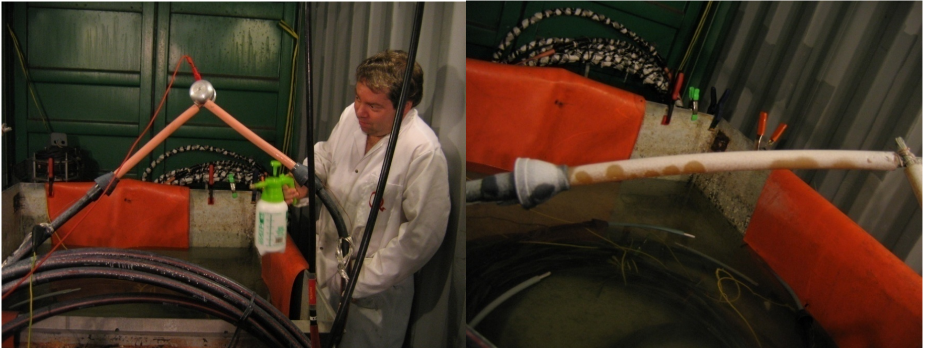
Normal clean test terminations prior to pollution
