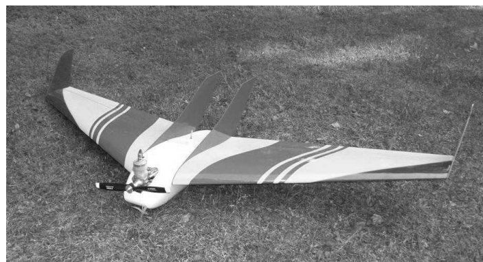
Fig.2. Miniature UAV prototype (developed in National Technical University of Ukraine “KPI”)
