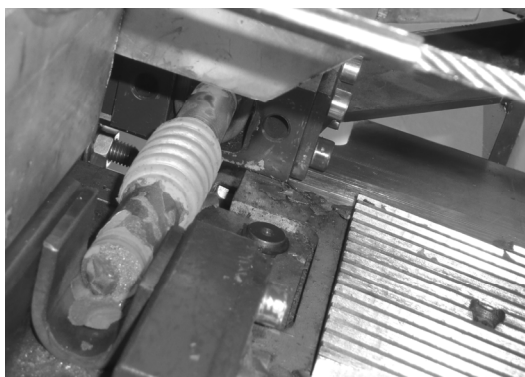
Fig. 6. The formed worm just after its winding has been rolled (a), sample worms produced by cross-wedge rolling with use of flat tools (b)
