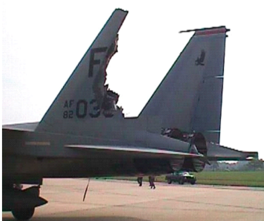
Figure 1: F-15 Damaged Vertical Tail; Consequence of Fatigue Damage Accumulation
