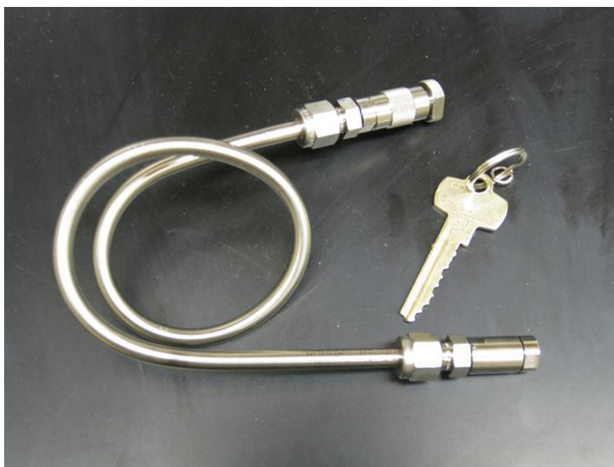
Figure 2.23: Photograph of the coiled continuous flow reactor.
