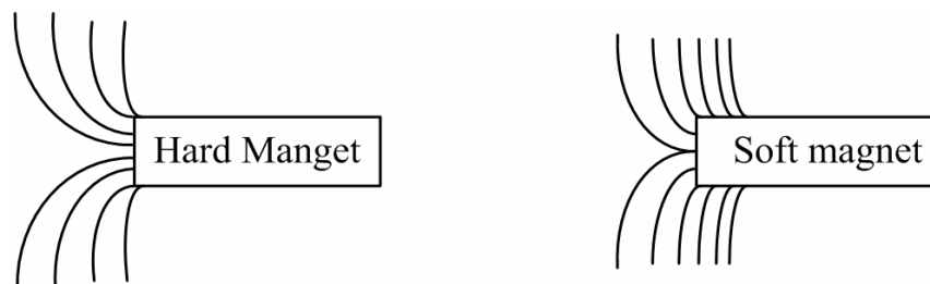
Figure 1-3 Comparison of Magnetic flux density distribution with different properties
