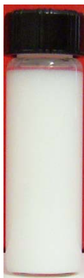
Figure 6.3 Stable ZnO/(polyacrylamide) nanocomposite latex prepared from the recipe in Table 6.2.
