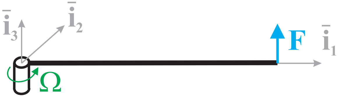
Figure 5.7: Rotating cantilevered beam subjected to transverse tip force.
