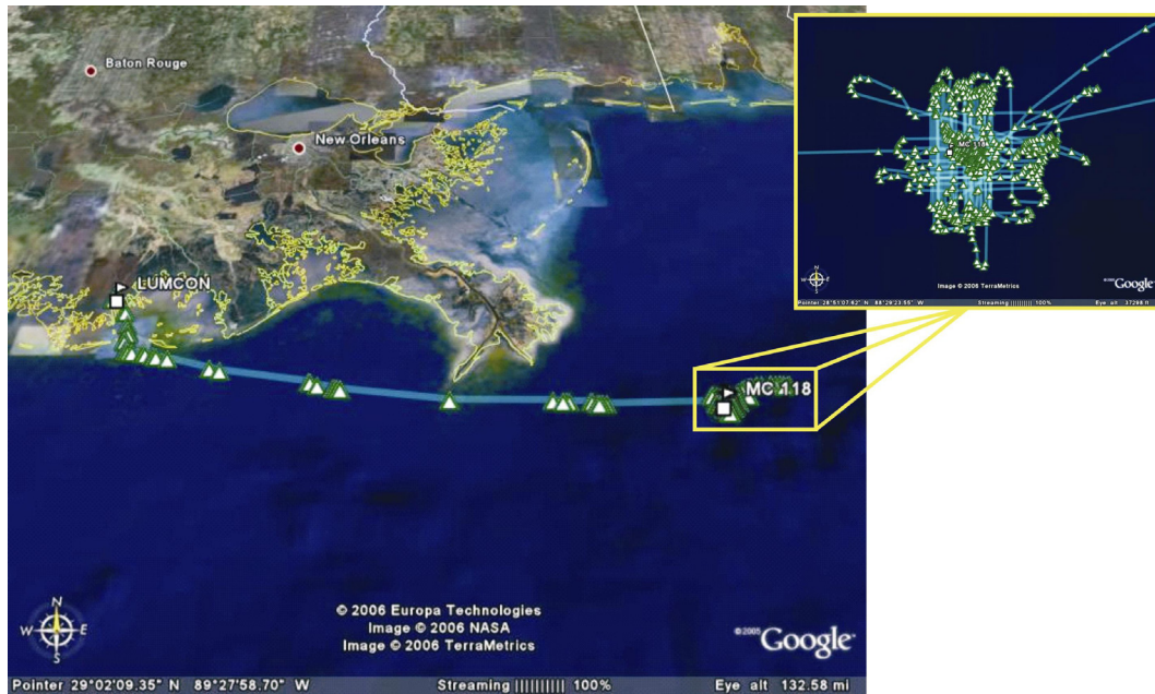
Figure 5-2: GPS trace of the June 2006 GOMGHRC cruise to MC118 aboard the R/V Pelican. The inset provides an accentuated view of grid profiles from the collection of geophysical lines for mapping acoustic reflections throughout the sediments.
