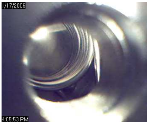
Figure 3-9: Optical image of the internal cooling coil inside the sample chamber as visualized through the optical viewport and captured by the hydrate imaging system.
