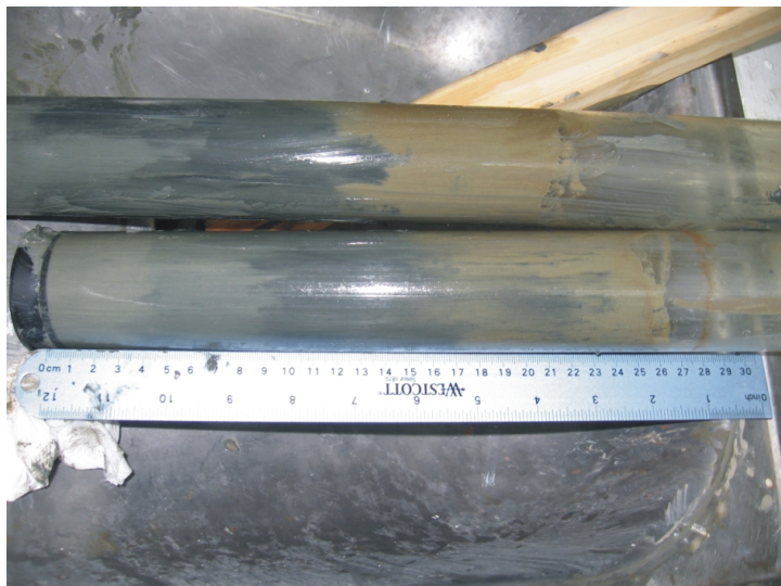
Figure 5-5: Representative image of a push-cored sub-sample with a 5.1 cm id. clear PVC pipe capped with rubber stoppers. Four distinct color changes within the sediments can be visualized in the pipe section next to the graduated ruler. The light brown layer in this image corresponds to the top sediment layer at the sediment-seawater interface.
