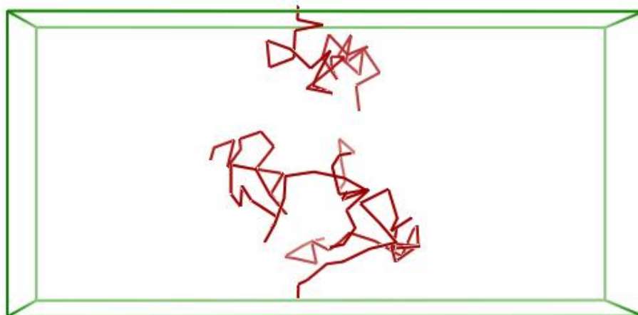
Figure 83: Polymer simulation using a bond spring constant of 5 and an equilibrium bond length of 10r_c .
