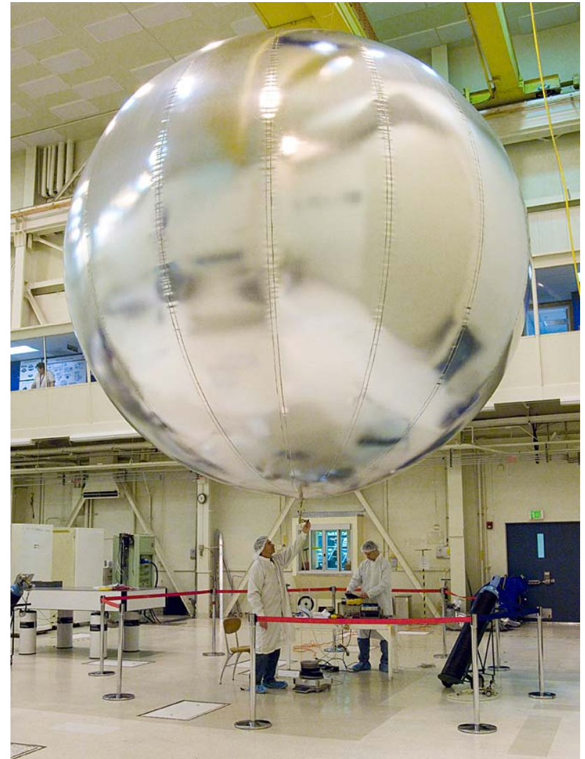
5.5 m diameter balloon prototype testing
