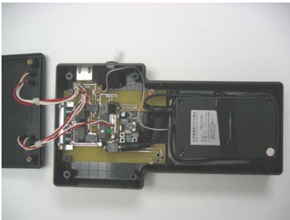
Figure 84: Battery and Power Switch Installed
