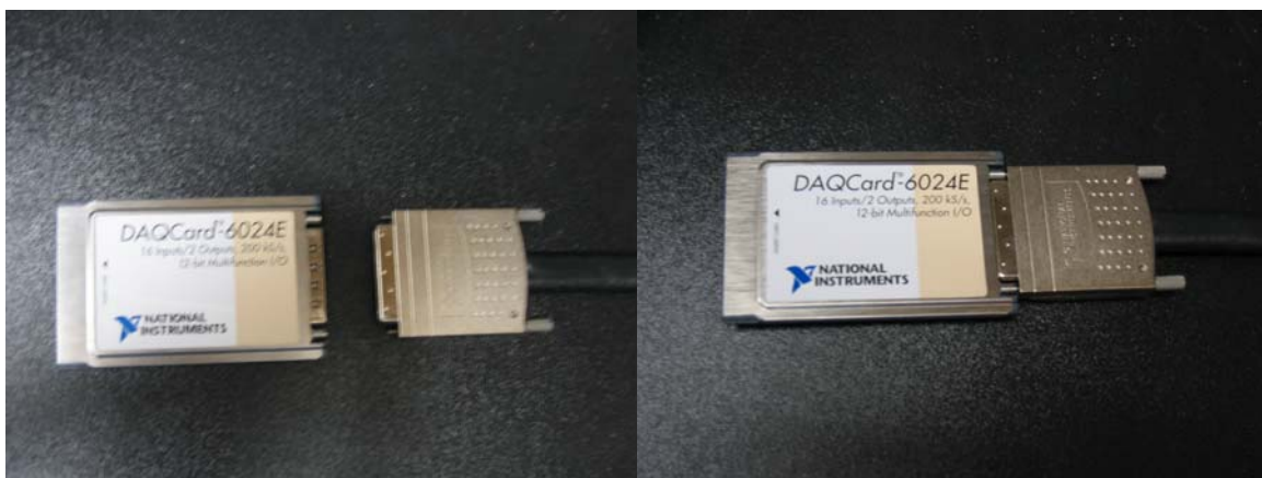
Figure 89: DAQ Cable connecting to PCMCIA card
