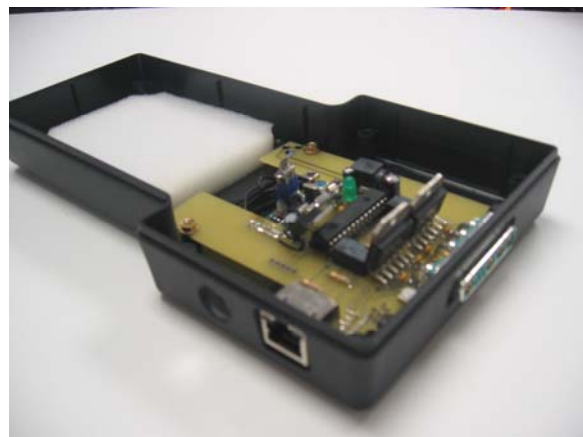
Figure 82: PCB Mounted Within Enclosure
