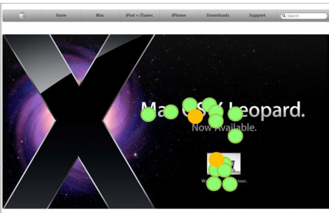
Figure 2.1. A user's gaze, demonstrating scanning and inspection behavior. Yellow circles represent entry points. Green circles represent inspecting fixations around the entry point.
