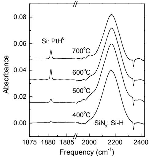
**Figure 2.** IR spectra for a bulk Si:Pt sample with a SiN<sub>x</sub> layer deposited on its surface by hot-wire CVD. The sample was annealed (10 min.) at the indicated temperatures to introduce H into the Si. Vibrational lines assigned to Si-H bonds in the SiN<sub>x</sub> layer and to PtH complexes in the Si are shown.
