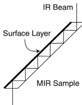
**Figure 1.** Multiple-internal-reflection geometry used for IR measurements of Si samples hydrogenated from a SiN<sub>x</sub> surface layer.
