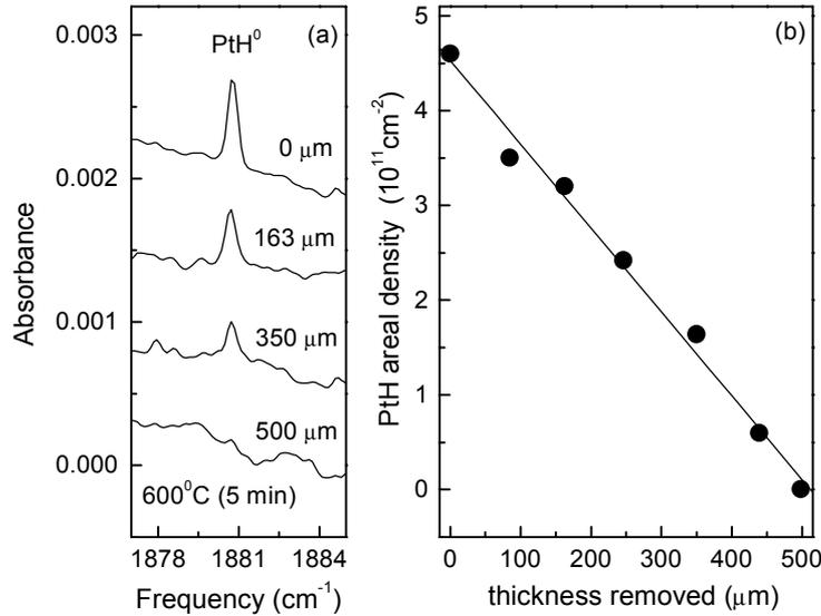
**Figure 3.** (a) IR spectra showing the vibrational line of the PtH complex in a Si:Pt sample that was hydrogenated by the post-deposition annealing (5 min at 600°C) of a PECVD SiN<sub>x</sub> film. Spectra were measured after a surface layer of the indicated thickness had been removed from the sample. (b) The areal density of PtH complexes remaining in the sample vs. the thickness of the layer removed from the surface, derived from the data shown in (a).
