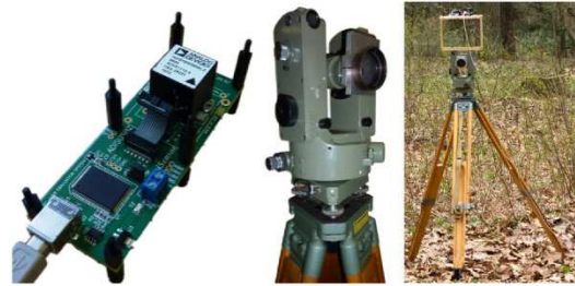
Fig. 3. The Inertial measurement unit ADIS16405 (on the left); theodolite T1c (in the middle); the whole measurement setup (on the right).
