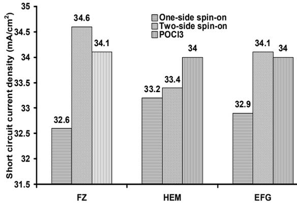
**Figure 2:** Short circuit current density as a function of material and type of emitter.
