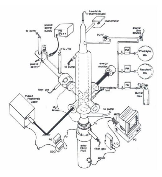
Figure 1. Schematic diagram of our Laser Flash Photolysis – Resonance Fluorescence (LFP-RF) apparatus [Finlayson-Pitts et al., 2000]
