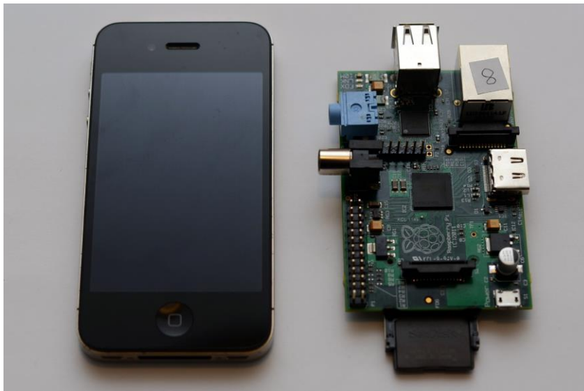
Figure 24 - Size comparison between a modern smartphone (left, iPhone 4s) and a Raspberry Pi (right, B+ model)
