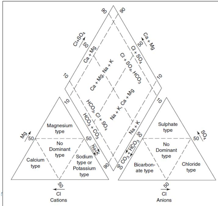
Figure 11. Exemplification of the Piper diagram showing hydrogeochemical classification for groundwater (Fetter, 2001).
