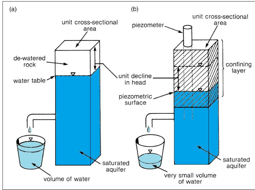
Figure 21. Diagrams illustrating storage coefficient for (a) unconfined aquifer and (b) confined aquifer (adapted from Brassington, 2007).
