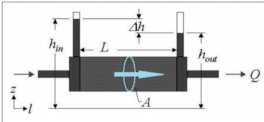
Figure 22. Schematic illustrating steady flow through a sand sample (Ahmed et al., 2008).
