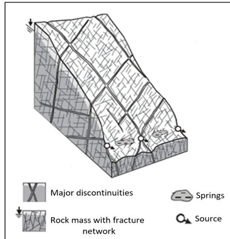
Figure 2. Conceptual diagram of a fractured rock mass aquifer (adapted from Pochon & Zwahlen, 2003).
