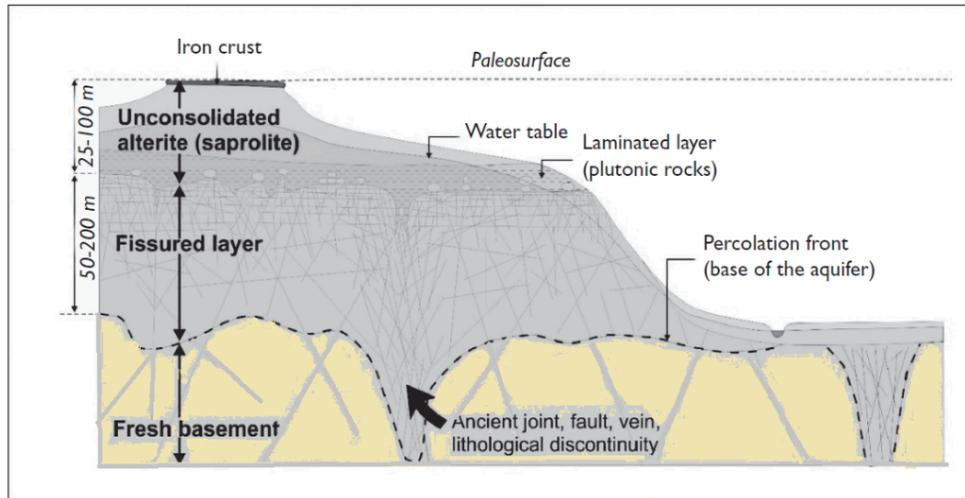
Figure 18. Stratiform conceptual model of the structure and the hydrogeological properties of hard rock aquifers (Sharp, 2014).
