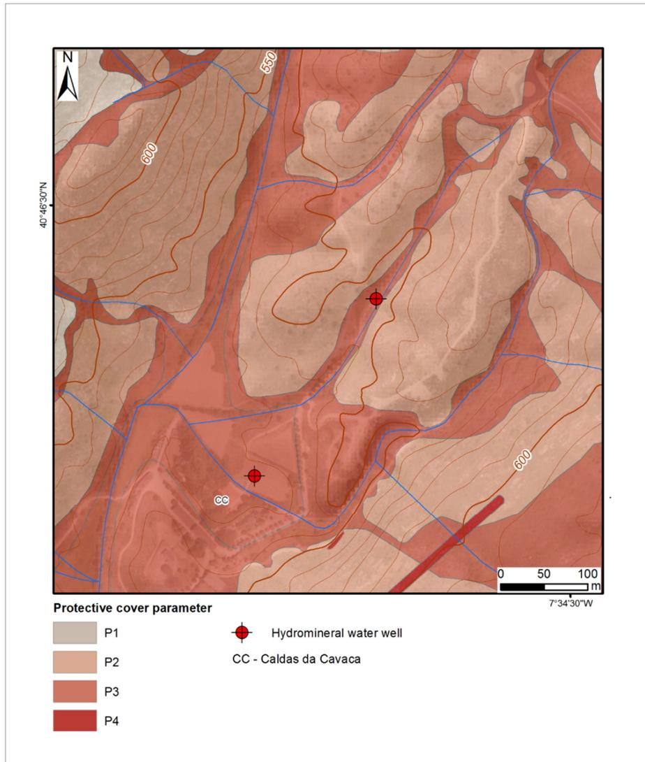
Figure 50. Map of the protective cover parameter for the hydromineral water wells (Caldas da Cavaca site).
