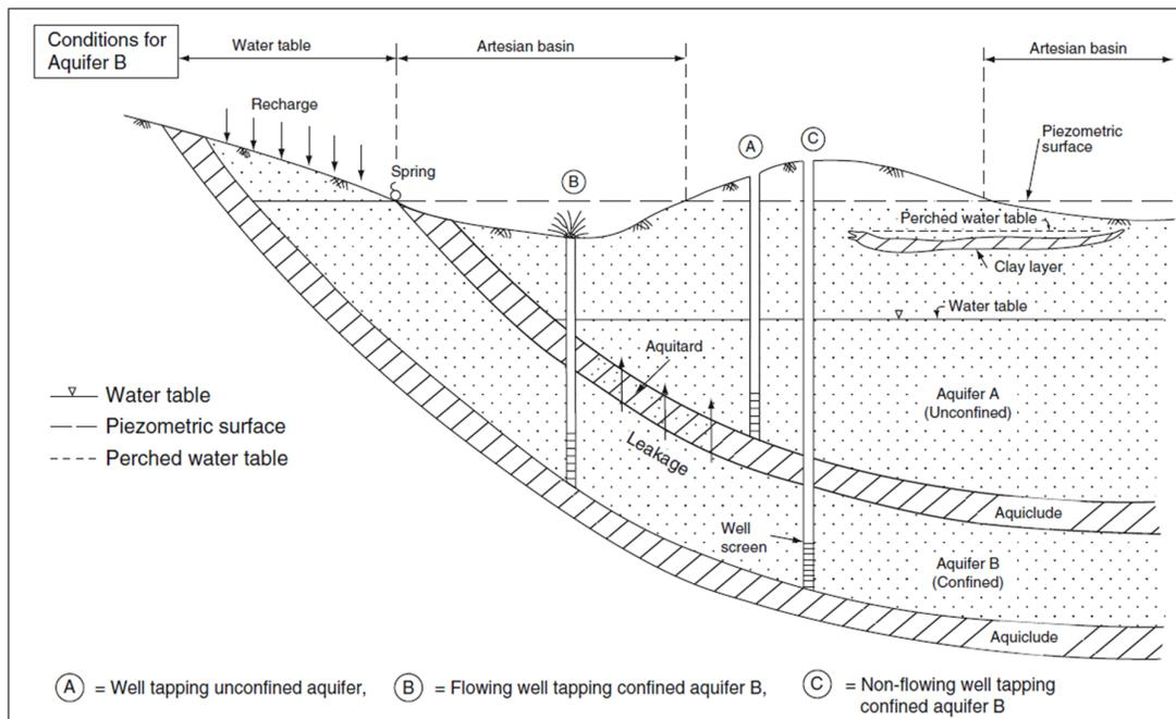
Figure 13. Types of geological formations. (A) Well tapping unconfined aquifer. (B) Flowing well tapping confined aquifer B, (C) Non-flowing well tapping confined aquifer B (Singhal & Gupta, 2010).
