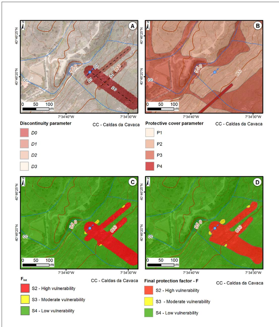
Figure 53. DISCO method applied to a spring at Caldas da Cavaca site: a) discontinuity parameter; b) protective cover parameter; c) intermediate protection factor ( $F_{int}$ ); d) Final protection factor (F).
