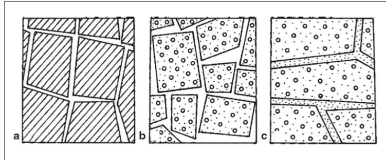
Figure 17. Schematic representation of (a) purely fractured medium, (b) double-porosity medium, and (c) heterogeneous medium (Singhal & Gupta, 2010).
