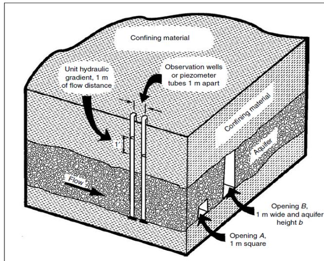
Figure 20. Diagram illustrating transmissivity (T) and coefficient of hydraulic conductivity (K). Flow of water through opening A will be equal to K and that through opening B equal to T (Delleur, 2007).
