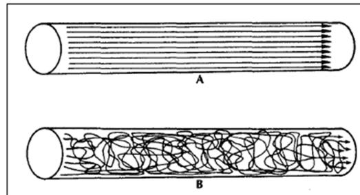
Figure 23. Schematic representation of laminar flow (A) and turbulent flow (B) (Sterrett, 2007).
