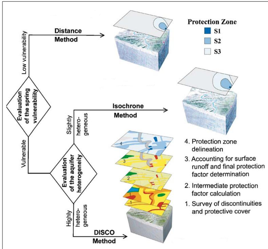
Figure 7. Decision process allowing the selection of one of three specific methods to delineate groundwater protection zones in fractured media (Pochon et al., 2008).
