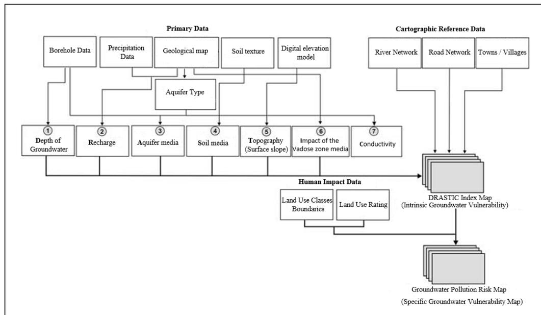
Figure 34. Schematic representation of the processes used to determine DRASTIC intrinsic vulnerability map and groundwater pollution risk map (Panagopoulos et al., 2005).
