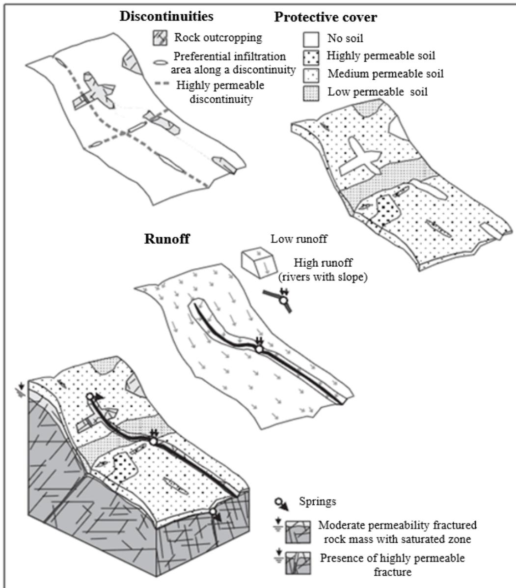
Figure 37. Representation of the three parameters considered in the DISCO method (adapted from
