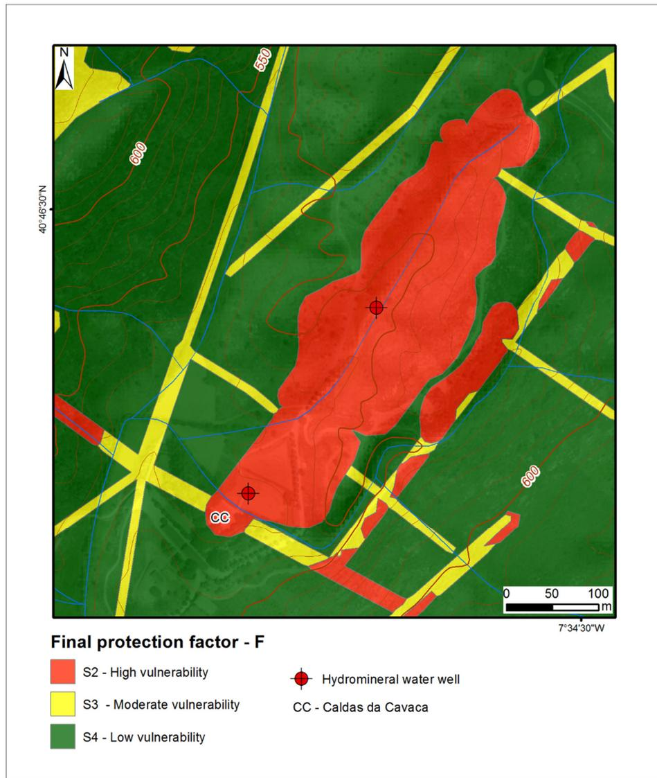
Figure 52. Map of the final protection factor for the hydromineral water wells (Caldas da Cavaca site).
