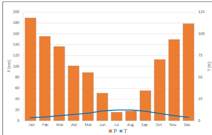
Figure 41. Thermo-pluviometric diagram concerning climatological station of Aguiar da Beira. (P) Precipitation; (T) Temperature (adapted from Teixeira, 2011).
