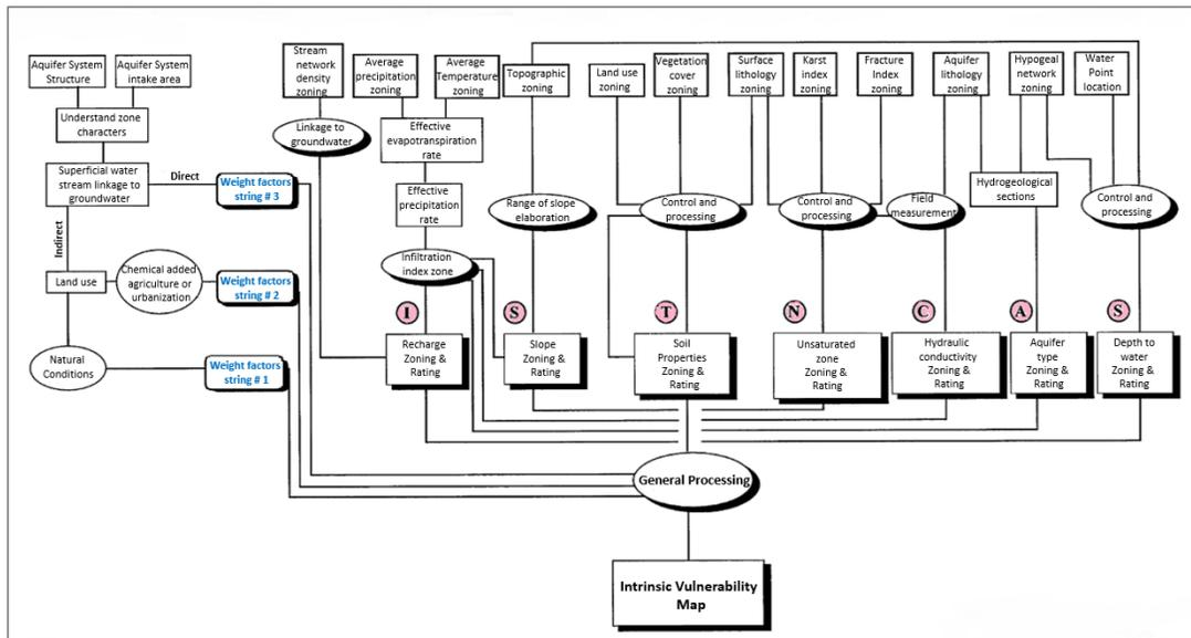
Figure 36. Schematic representation of the steps of SINTACS method (Gogu & Dassargues, 2000).
