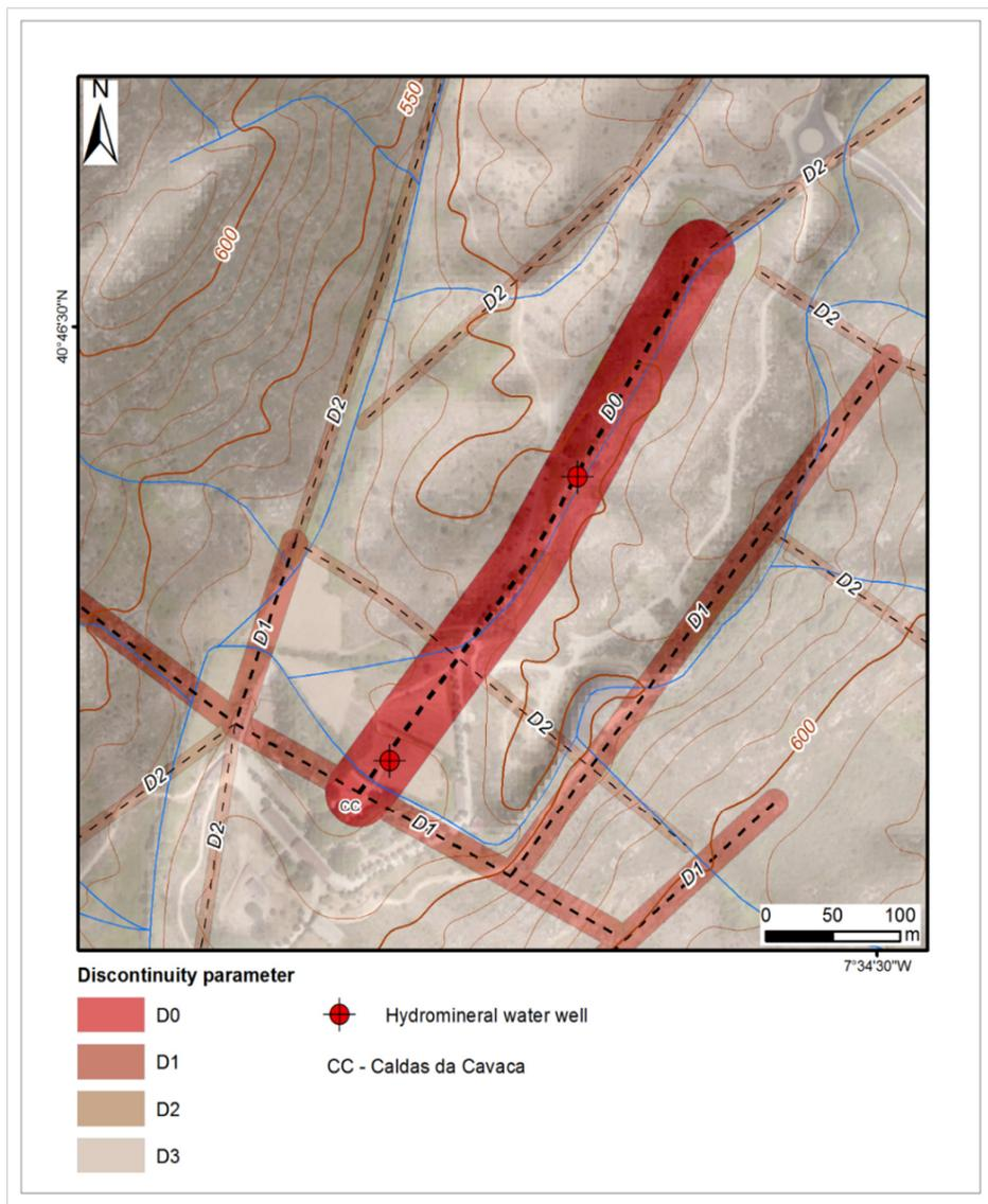
Figure 49. Map of the discontinuities parameter for the hydromineral water wells (Caldas da Cavaca site).
