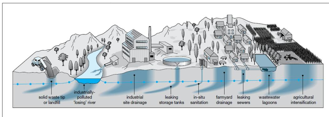
Figure 24. Common processes of groundwater pollution (Foster et al., 2002).
