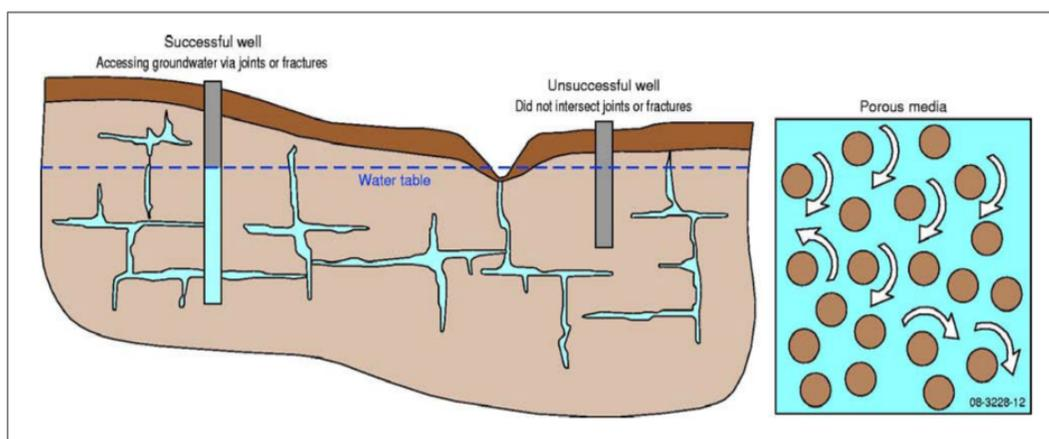
Figure 16. Comparison of groundwater systems in fractured aquifers (left) and porous media (right) (Lewis et al., 2008).
