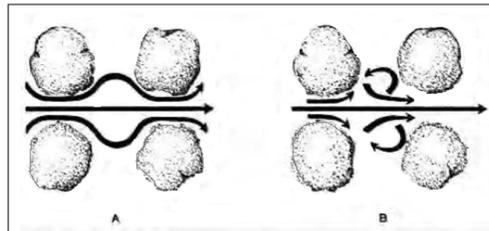
Figure 4. Flow paths of molecules of water. A: in laminar flow; B: in turbulent flow (Fetter, 2001).
