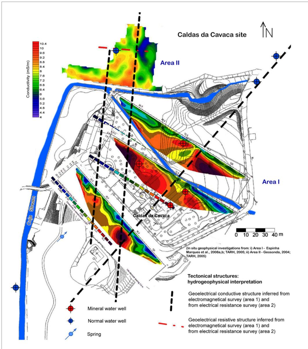
Figure 46. Synthetic interpretation of geophysical surveys in the area of Caldas da Cavaca (updated from Teixeira, 2011).
