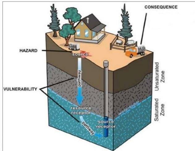
Figure 26. Source–pathway–receptor model for contaminants (NRC, 2005).
