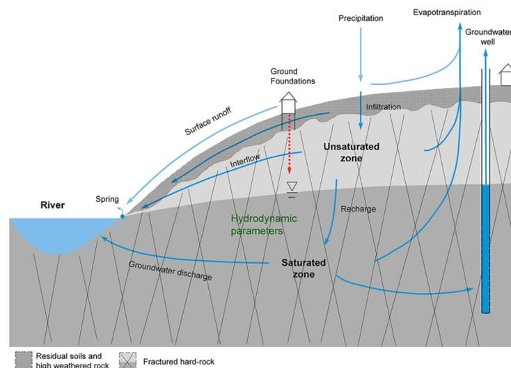
Figure 1. Schematic diagram of the hydrological cycle in a hard rock fissured framework (Fitts, 2013; adapted from Chaminé et al., 2013).
