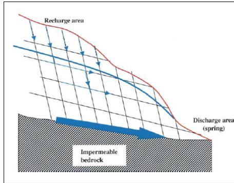
Figure 3. Diagram of the flow condition typical of a rock slope with an impermeable bedrock with indication of the water flow direction within the discontinuity network (Scesi & Gattinoni, 2009).
