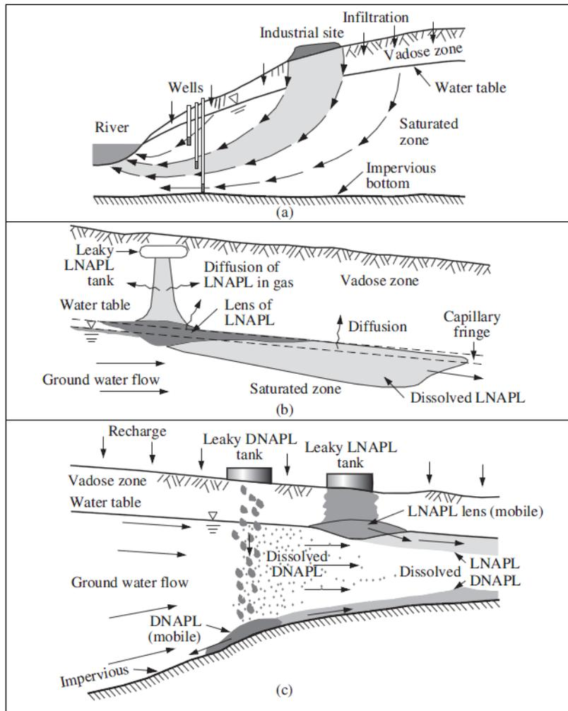
Figure 25. Typical cases of subsurface contamination (Bear & Cheng, 2010). (a) The migration of a contaminant that is leached from a landfill: the leachate travels through the vadose and then through the (saturated) aquifer, eventually draining to a river; (b) An LNAPL leaks from an underground storage tank and migrates through the vadose zone, eventually accumulating on an underlying water table; (c) Different routes through which a DNAPL and an LNAPL can contaminate an aquifer.
