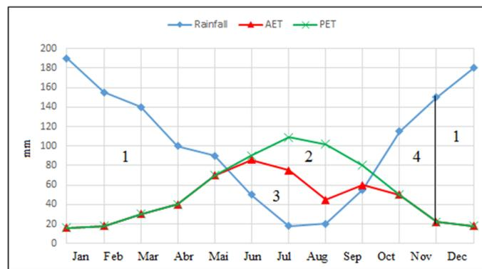
Figure 42. The annual water balance of Caldas da Cavaca area: 1- Water surplus; 2- Water deficit; 3- Soil moisture storage withdrawal; 4- Soil moisture storage increase; PET- Potential Evapotranspiration; AET- Actual Evapotranspiration. (adapted from Teixeira, 2011).
