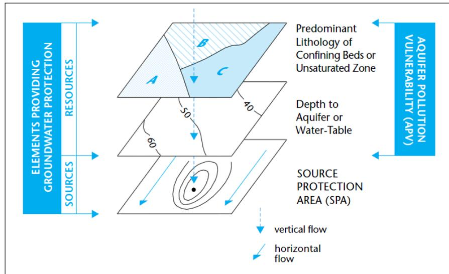
Figure 29. Components of groundwater pollution hazard assessment used for groundwater protection land surface zoning (Foster et al., 2002).
