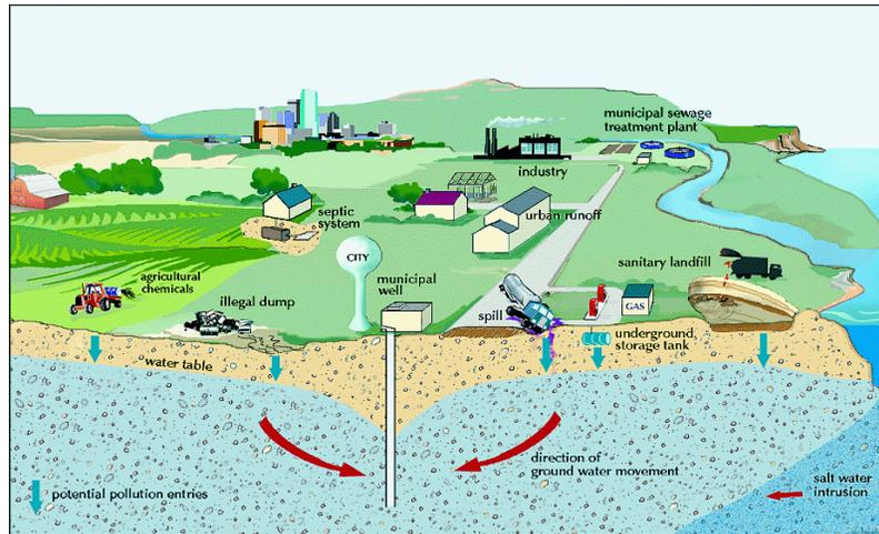
Figure 5. Schematic overview of the main sources of groundwater contamination (Zaporozec, 2004).
