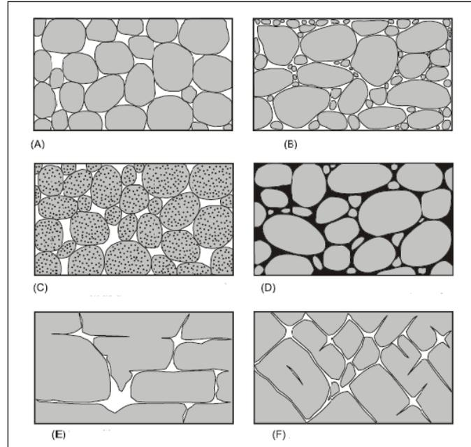
Figure 19. Porosity of typical aquifer materials. (a) Good rating sediments have a high porosity. (b) Poor rating sediments have a low porosity. (c) The grains are porous, so increasing the overall porosity of the formation. (d) The porosity is often reduced by the existence of cementing material. (e) Rock with porosity increased by solution. (f) Rock with porosity increased by fracturing (Brassington, 2007).
