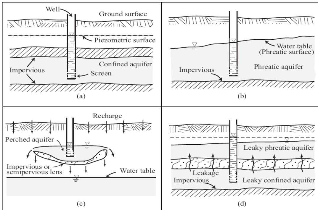
Figure 15. Types of aquifers: (a) Confined aquifer; (b) Phreatic aquifer; (c) Perched aquifer; (d) Leaky aquifer (Bear & Cheng, 2010).
