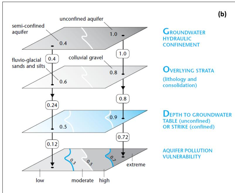
Figure 31. (a) GOD system for evaluation of aquifer pollution vulnerability; (b) Generation of aquifer pollution vulnerability map using the GOD system (Foster et al., 2002).
