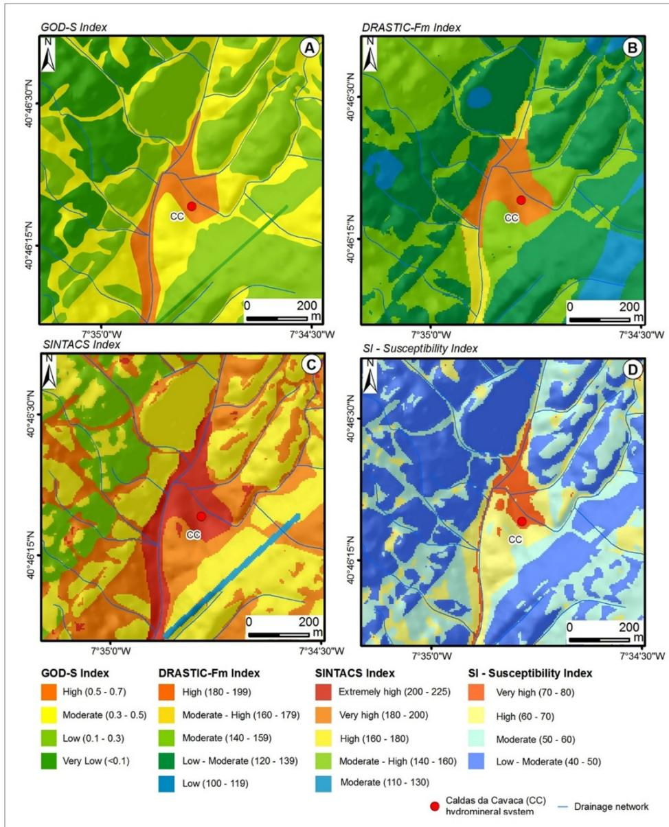
Figure 47. Vulnerability indexes from Caldas da Cavaca aquifer systems and surrounding area: a) GOD-S; b) DRASTIC-Fm; c) SINTACS; d) SI (updated from Teixeira et al., 2015).
