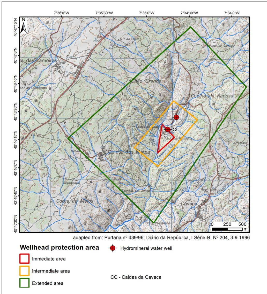
Figure 54. Wellhead protection areas defined in 1996 for Caldas da Cavaca spa.
