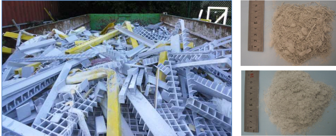
Fig. 3 Typical wastes of GFRP pultrusion process (left) and samples of obtained recyclates after mechanical recycling in a heavy-duty cutting mill using different sized-meshes inside the grinding chamber (right).
