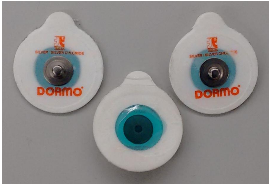
Figure 20 – Top and bottom view of electrodes used in EMG.
