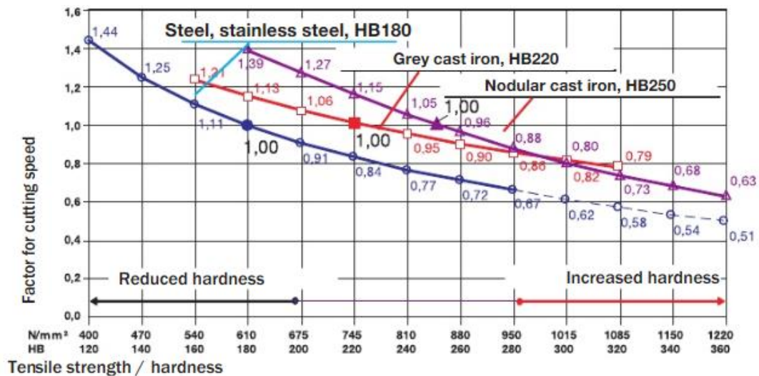
Figure 2-27. Diagram comparing the hardness and factor for cutting speed [59].
