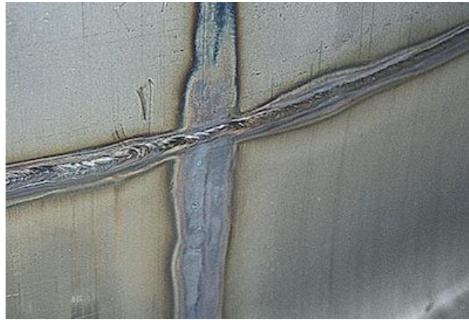
Figure 2-35. A heat tinting that shall be removed and the easiest way to do this is by pickling process [65].
