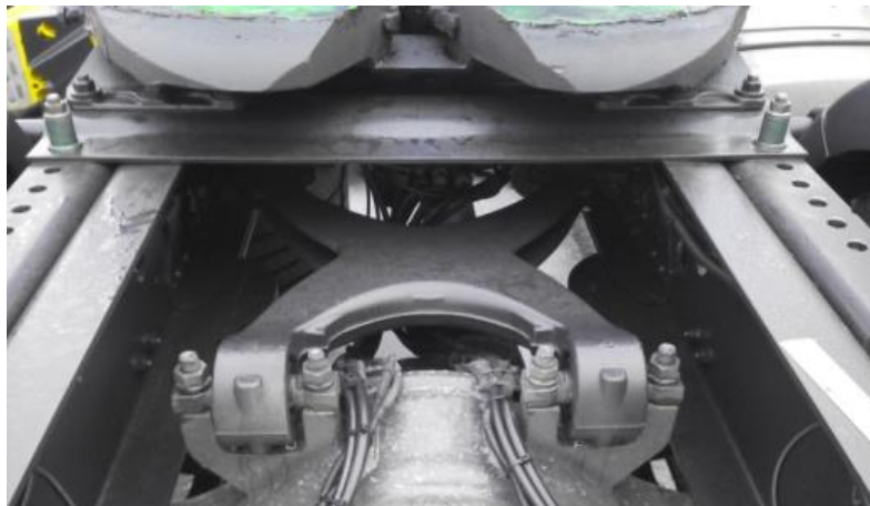
Figure 3-9. X-link used on heavy duty MAN TGA truck. It ensures the directional and vehicle stability and damping control.
