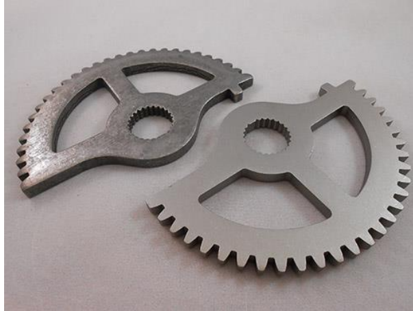
Figure 2-33. Component before (to the left) and after (to the right) shot peening [81].
