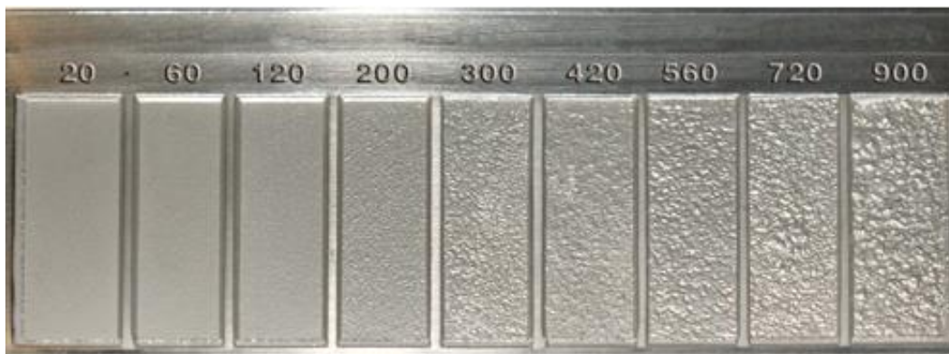
Figure 2-9. C-9 microfinish comparator [26].
