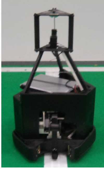
Fig. 3. 5dpo soccer robot with a catadioptric vision system (left). SocRob soccer robot with a dioptric vision system (right).
