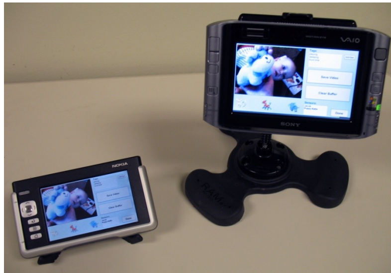
Figure 31: KidCam shown with remote monitoring device on Nokia 770 shown to the left of it.
