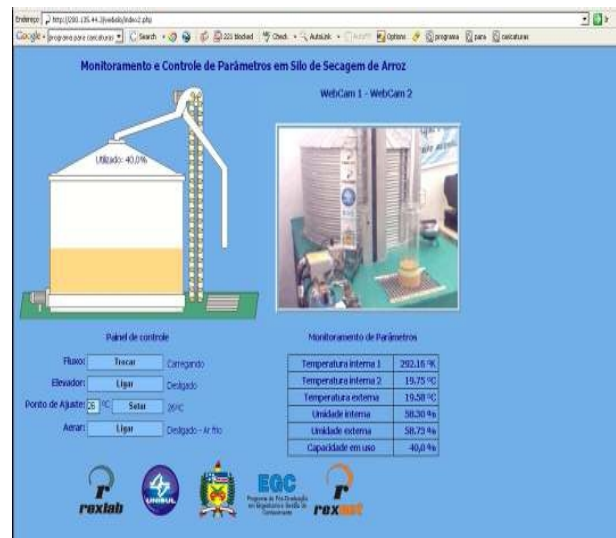
Fig. 7: Web page for controlling and monitoring the silos model.
