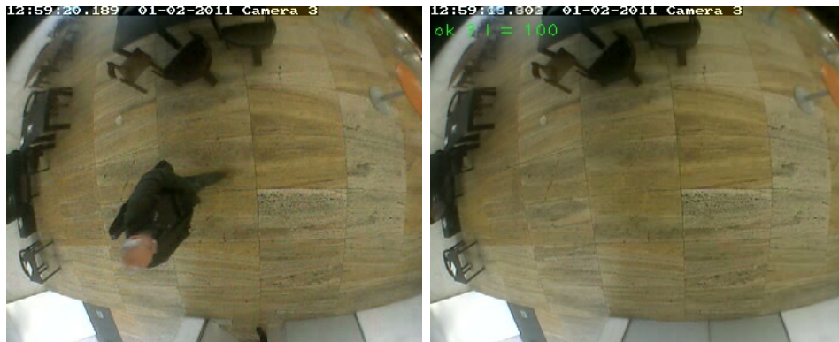
Figure 5.3: Sample image processing from Background Estimation Module: left - Original Image; right - Background Average.
