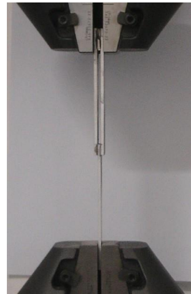
Fig. 4. Double-lap joint with L_o \frac{1}{4} 10 mm in the testing machine under testing.
