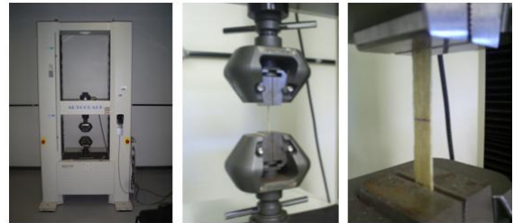
Figure 3. Tensile test for sisal fibre composite.
