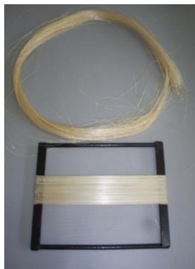
Figure 1. Assembly of natural fibres using a metallic structure
