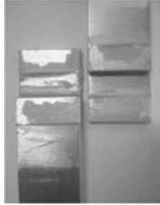
Figure 17. Example of adhesive failure for a DS repair with L_O = 10 mm (without plug-filling).
