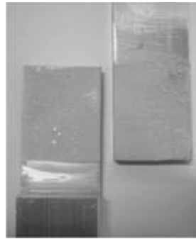
Figure 7. Example of cohesive failure for a SS repair with L_O = 30 mm (without plug-filling).
