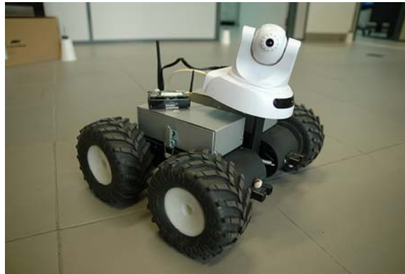
Figure 26- Intruder robot carrying a mote
