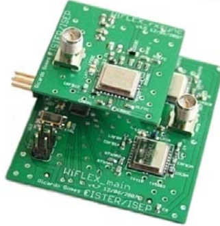
(c) WiFLEX_daughter board stacked on the WiFLEX_main board
