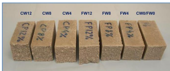
Fig. 3. Samples of broken PM test specimens after being tested in flexural (one sample of each CW and FW test series).
