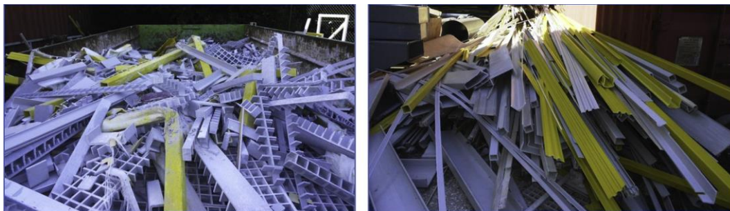
Fig. 1. Samples of production wastes and non-conform products of the pultrusion industry (courtesy of Alto, Perfis Pultrudidos Lda.).
