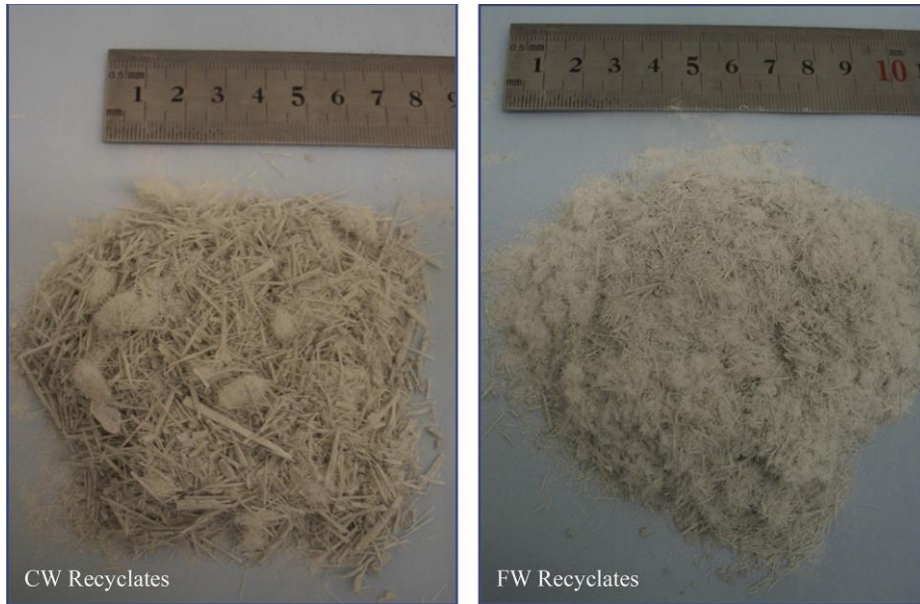
Fig. 3. Samples of CW and FW recyclates.
