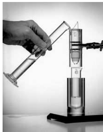
Figure 3 – Image representing the first Molybdenum-99 / Technetium-99m Generator, unshielded (1958). A Tc-99m pertechnetate ( ^{99m}\text{Tc} ) solution is being eluted from Mo-99 molybdate ( ^{99}\text{Mo} ), bounded to a chromatographic column.
