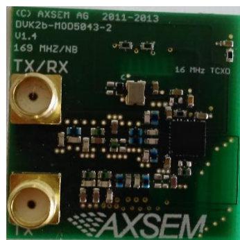
Figure 30 - AX5043 RF-ICs modules.
