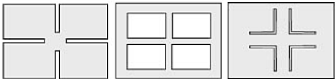
Figure 8: Examples of cuts in patch antenna [2]
