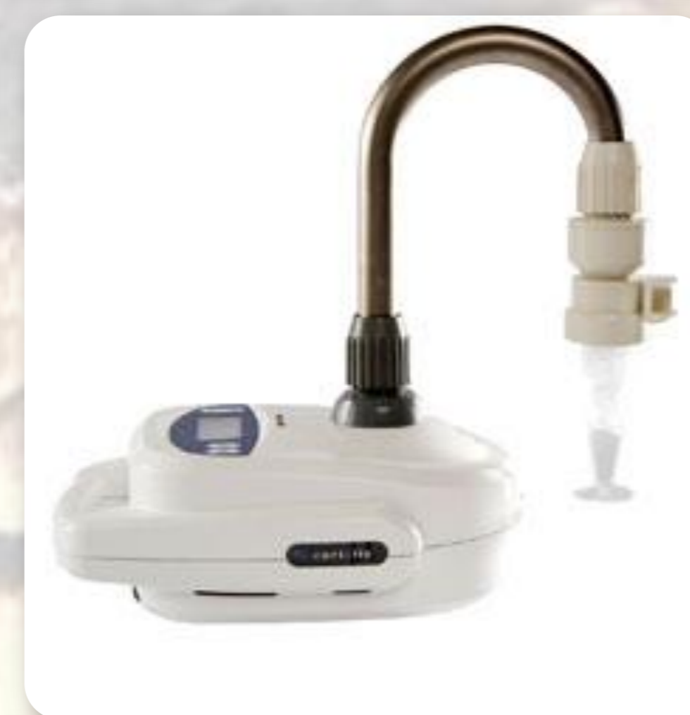
Fig. 3 - Equipment used for air samples collection through impinger method
