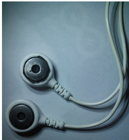
Fig. 4.12. Prototype ECG acquisition sensors.
