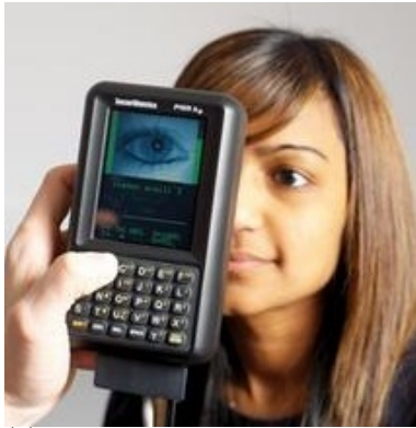
(a) Iris scanner for person identification [5].
