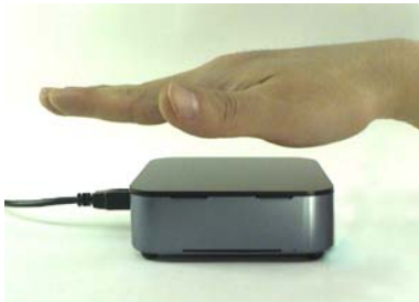
(c) Over air hand palm scanner [7].
