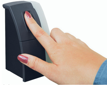
(b) Fingerprint scanner for restricted accesses [6].
